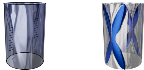
Fig. 6. Cylinder with top and bottom nodes fixed and pulling force (100 N) distributed on two sides. Left: the initial deformation before topology optimization with boundary condition marked in black. Right: the optimized structure.
