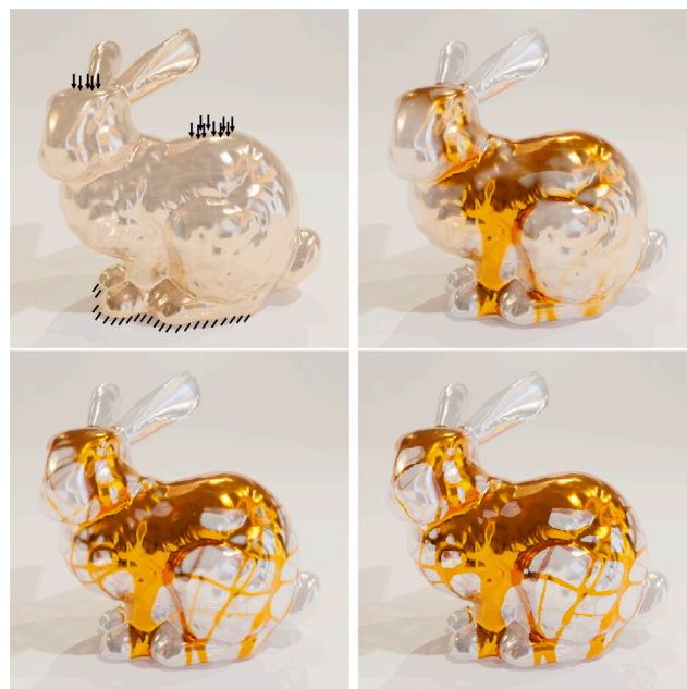
Fig. 12. Optimization intermediate states of the Stanford bunny at iteration 1, 20, 100 and 250. The boundary condition is indicated in the first picture, where the bottom nodes of the bunny are fixed and loads are applied on the head and the back.
