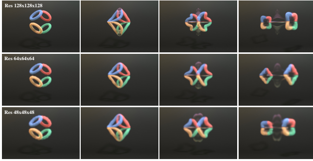
Fig. 4. Four-Vortex Collision. We simulate four colliding vortices as in [Matsuzawa et al. 2022]. The collision causes the vortices to merge into two star-shaped vortices, drifting toward opposite walls while altering their shapes. Our simulation can run at resolutions of 48, 64, and 128.
