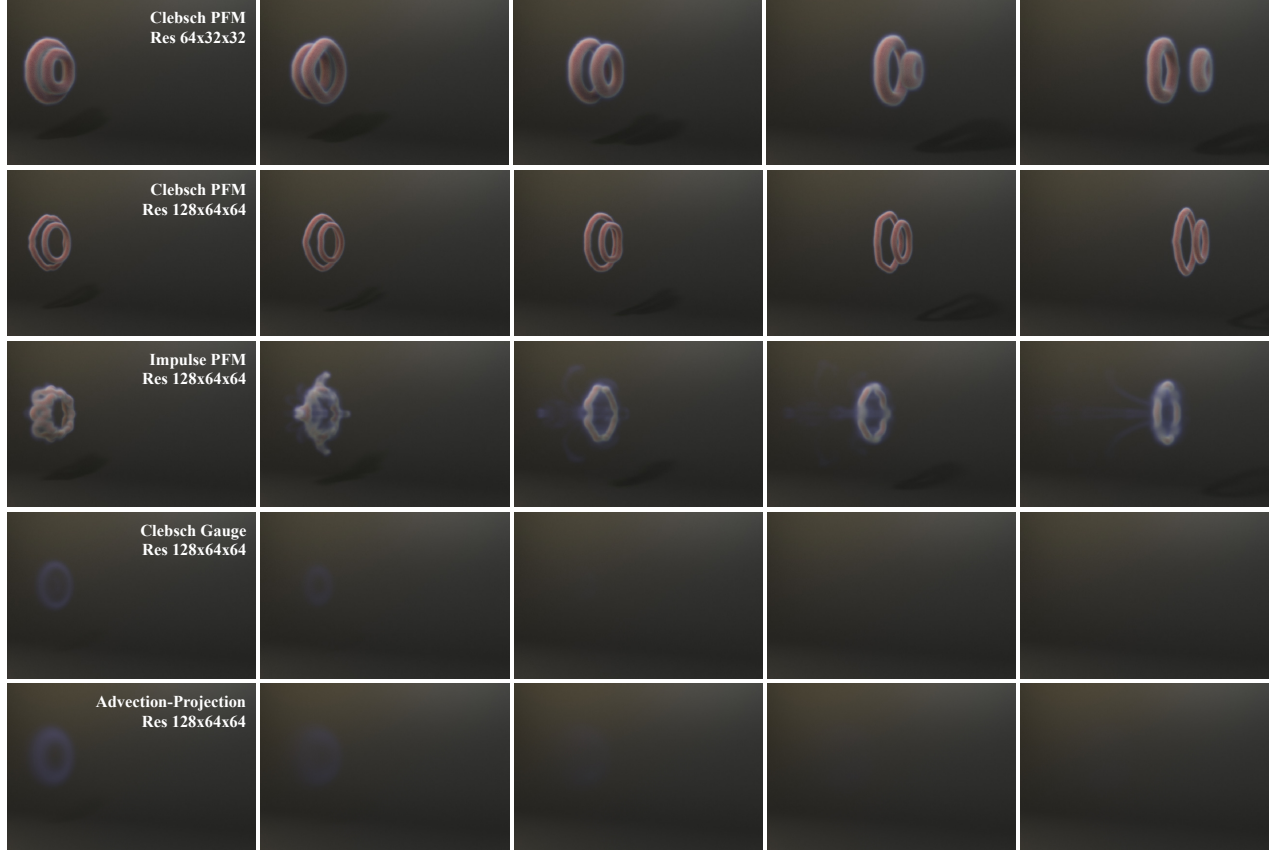
Fig. 12. Leapfrogging Vortices. In a 128 \times 64 \times 64 resolution, our method successfully maintains separation of the rings through six leaps and continues to sustain them for three leaps even when using a lower resolution 64 \times 32 \times 32 grid. In comparison, the impulse-based PFM results in merging after just one leap, while the Clebsch gauge method begins to lose vorticity following a single leap.
